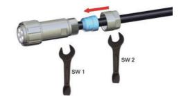
Insert sealing (3) completely and screw cap (2) onto basis (5).
